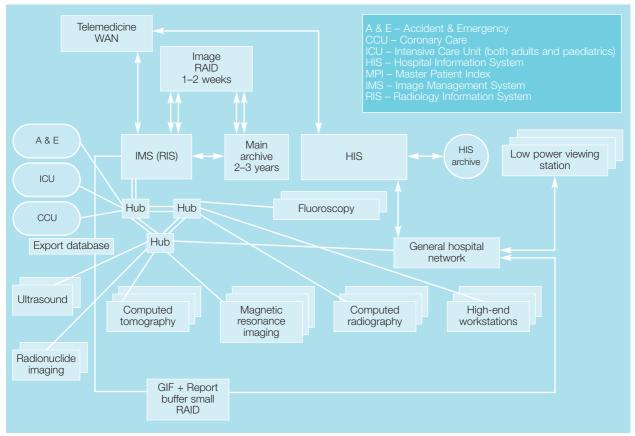
Figure 4.1 Basic conceptual diagram of proposed PACS/RIS and HIS integration
