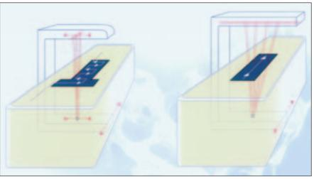
Figure 2.1 The scan configuration between a narrow-angle fan beam system and a conventional fan beam unit, courtesy GE
