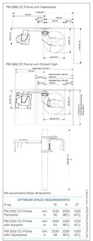
Figure 1.5 Example dimensions of an OPG/dental panoramic unit fitted with cephalostat attachment, courtesy Planmeca
