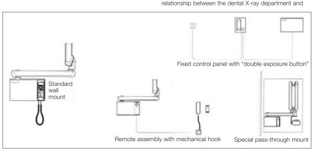
Figure 1.1 Examples of installation configurations for extra-oral dental units, courtesy Planmeca
