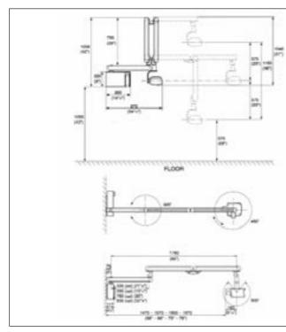
Figure 1.2 Example dimensions for a typical extra-oral X-ray unit, courtesy Planmeca
