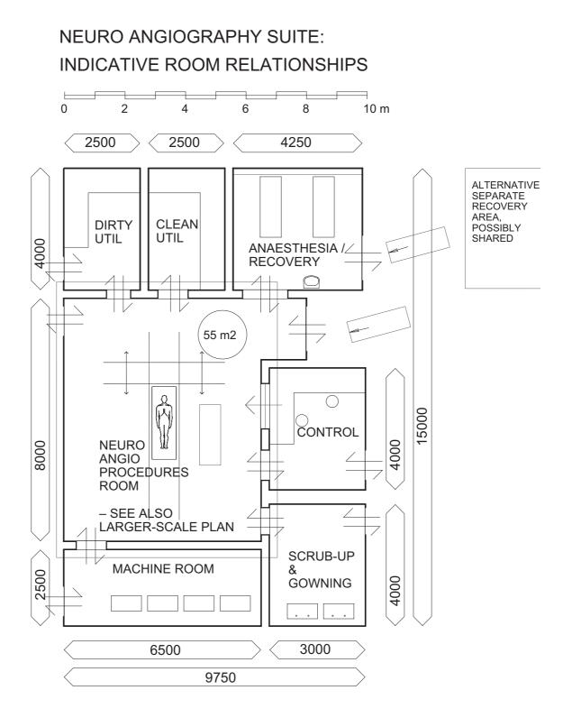
Note: this generic plan emphasises room layouts and adjacencies. It does **not** allow for other specific design requirements such as fire safety planning. Project and design teams must additionally consider such design factors, and adapt the generic plan accordingly.
