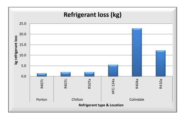
There is a legal requirement to monitor and measure the amount of refrigerants (known as F-gases) that are lost to the atmosphere from the operation of cooling and air handling systems fitted on our owned estate. At each of our properties where this
